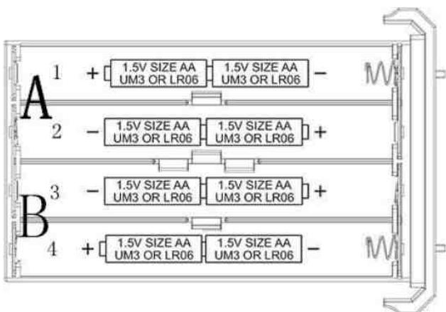
The working voltage of the camera is 12V. To supply power for the camera, 8 AA batteries are needed.
